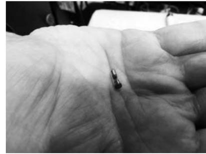
図3 Integrated Sensing Systems Inc.の無線機能付き体内埋込み心房圧測定用圧力センサ
